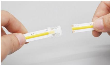
Insert each ends of led strips into the end of the connection terminal respectively, make sure the metal clip is on the same side as the metal solder pad of led strip.
