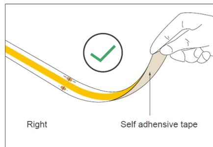
If the led strip needs to be torn up, please make sure that the self adhesive tape is torn with the led strip, otherwise the led strip will be damaged.
